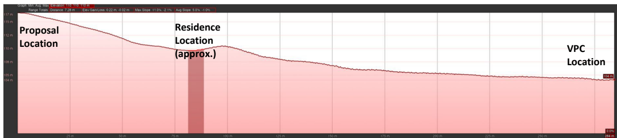
Figure 20 - VPC – Elevation profile from viewpoint to proposal showing that elevated topography does not block views of the proposal (Source: Google Earth).
